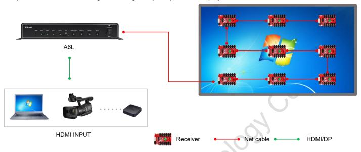
4. Multi-screen splicing application: use HDMI high-definition signal lines to splice in series, and automatically splice the contents of multiple display screens into an overall picture.
